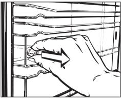
Pull on the fixing knob to release it.
